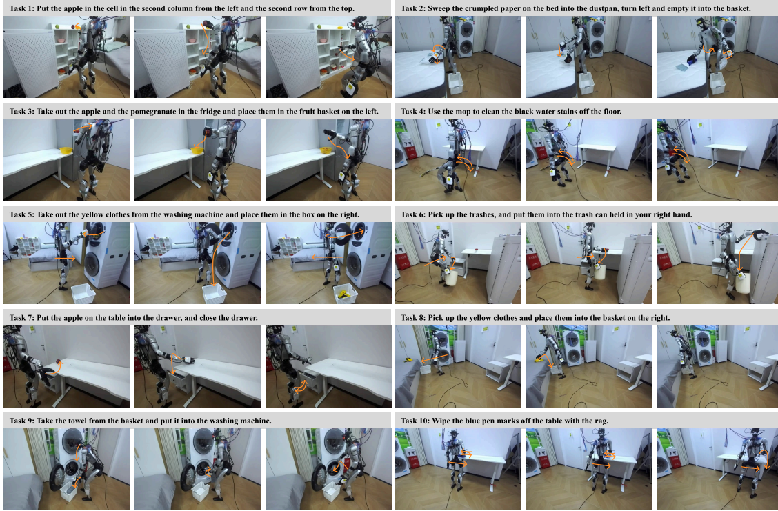
Figure 6 Real-world task setup. We evaluate \omega -0 on diverse long-horizon household loco-manipulation tasks involving whole-body motion, locomotion, tool use, articulated-object interaction, and dexterous manipulation. The task instruction is overlaid on each rollout sequence, and key sub-task progress is denoted with orange markers for better visualization. All rollouts are autonomously executed by the learned policy on the real humanoid.
