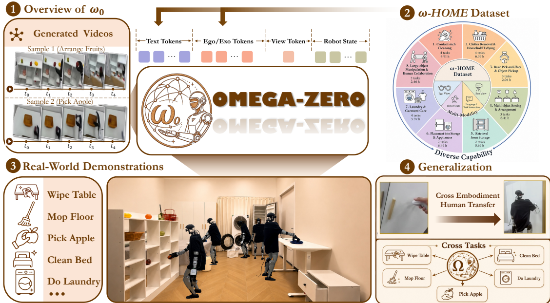
Figure 1 Overview of \omega -0 and the \omega -HOME dataset. \omega -0 generates whole-body action latents from language, multi-view observations, and robot states, while \omega -HOME provides 40h of multimodal household humanoid demonstrations for training and evaluation.
